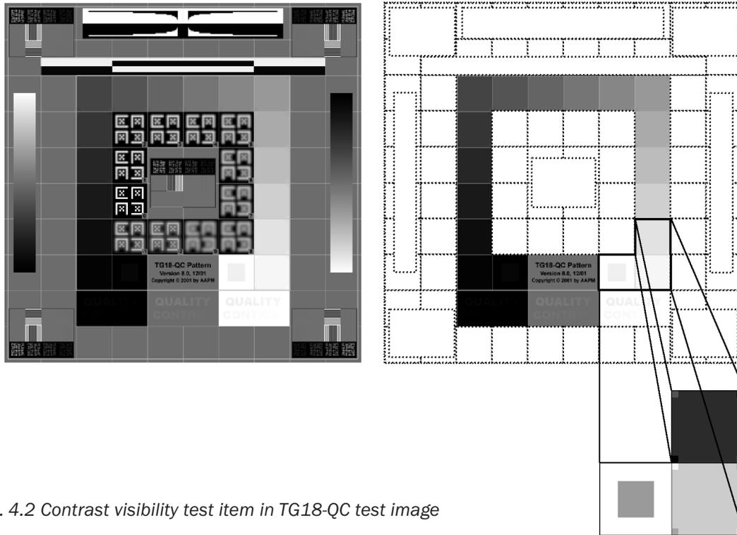
Fig. 4.2 Contrast visibility test item in TG18-QC test image
