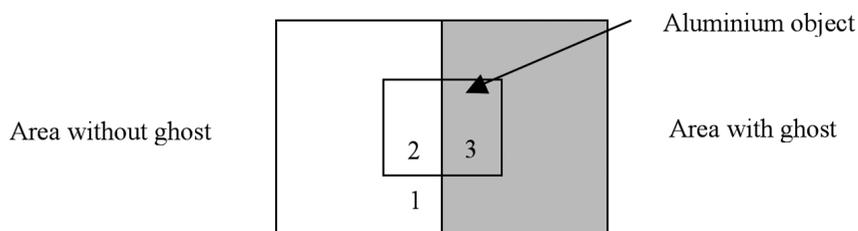
Fig. 2.2 Ghost image / erasure thoroughness measurement
